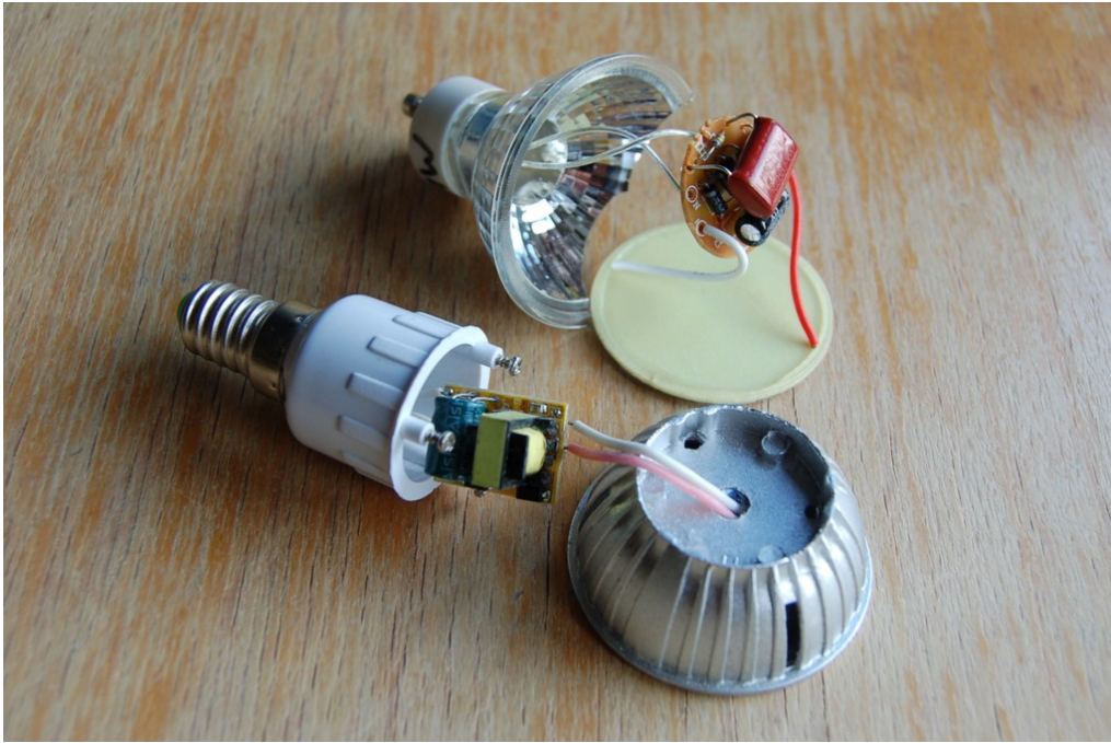
Figure 1: Front: EMI dirty LED bulb with unfiltered buck converter, recognisable by its yellow transoformer; Back: EMI clean LED bulb with a big, red-coloured series high-voltage capacitor.
