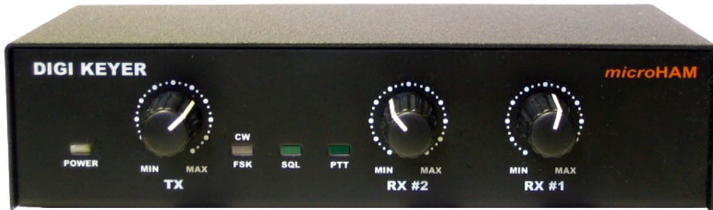
Figure 1: Front panel of the microHAM Digi Keyer
