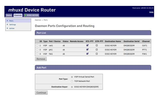
**Figure 3:** Configuration and routing of the mhuxd deamon virtual serial ports for the microHAM Digi Keyer
